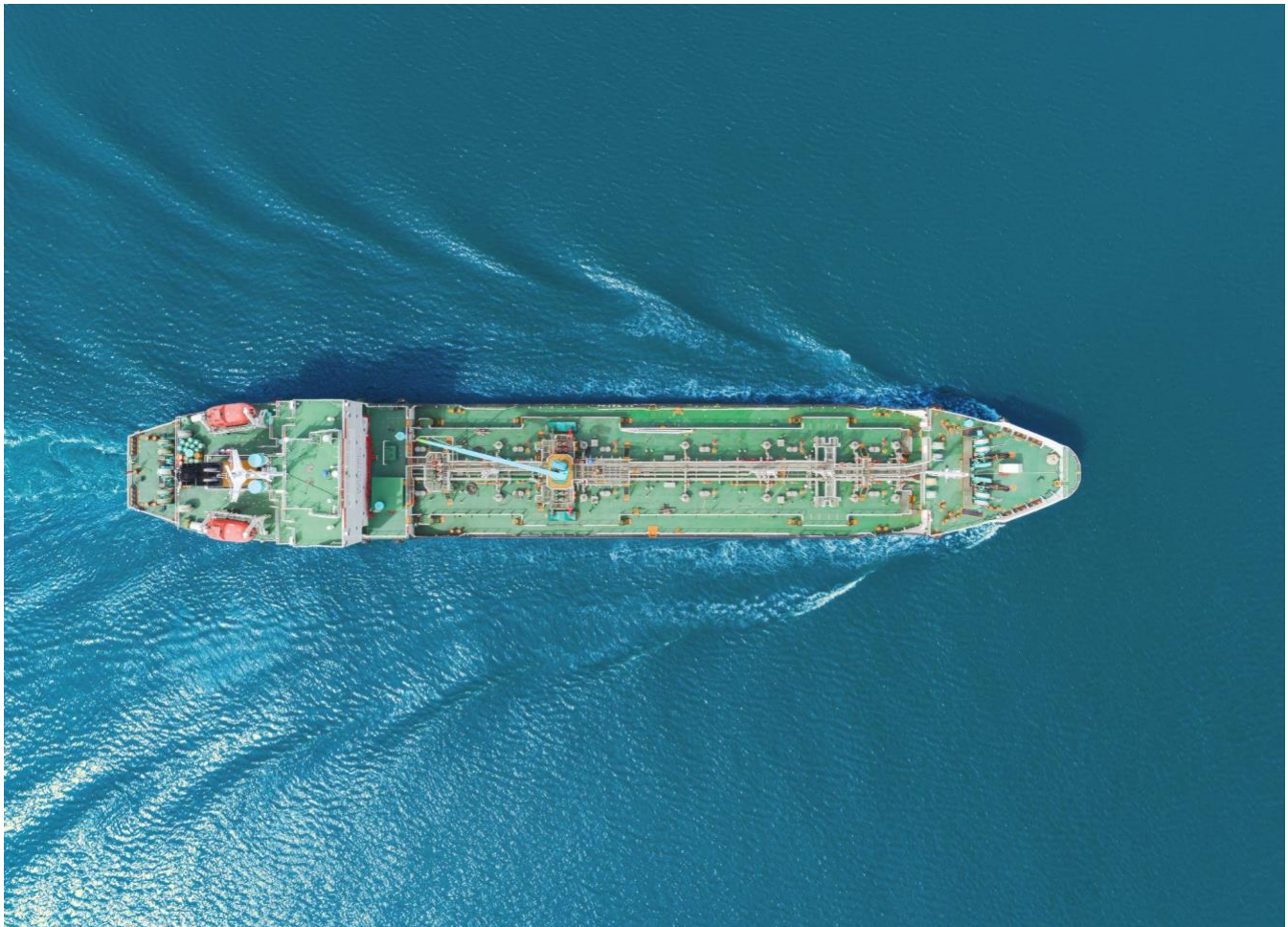
A Very Large Gas Carrier capable of transporting up to 60,000 tonnes of liquid ammonia.
